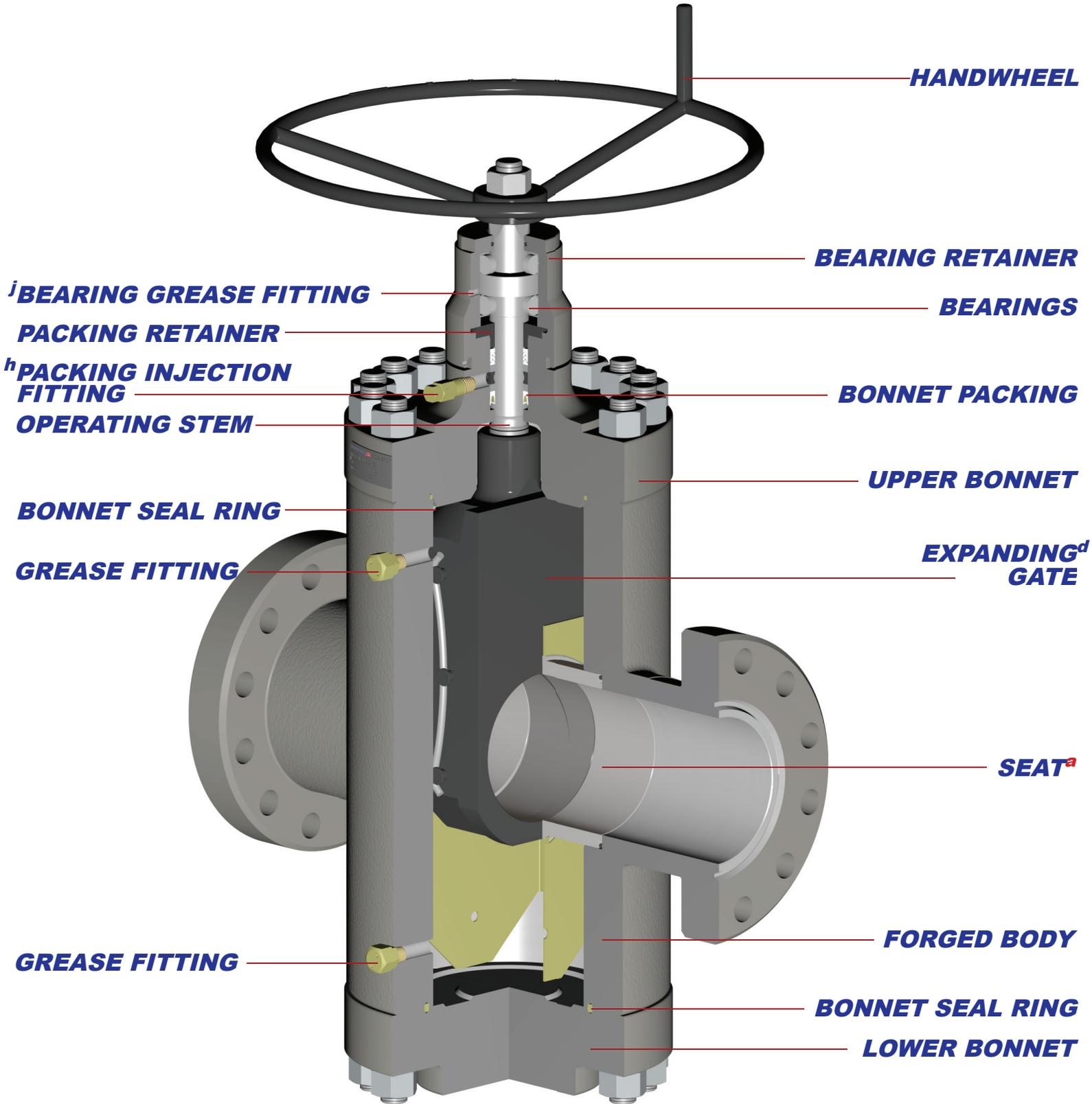
a) Equipped with a non-sealing seat on the upstream side. See engineering note titled "Model FM4 & Model FM4 RC" for details.
